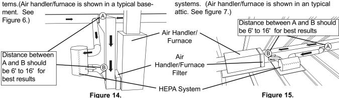
NOTE: This filtration system is an ADDITIONAL filter, and does NOT replace the existing air handler/furnace system filter.
